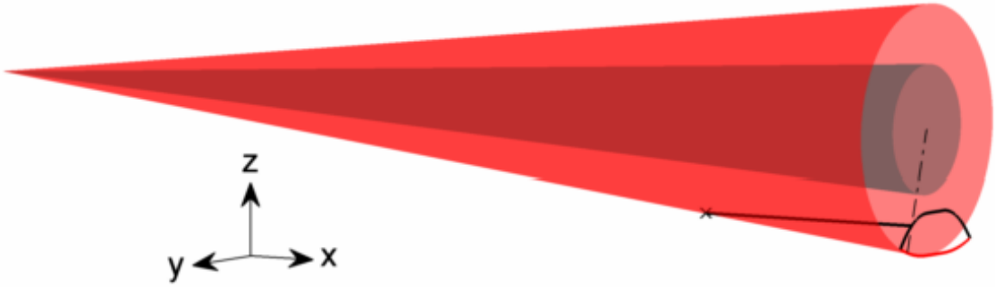
Figure 3.33: Moving directly upstream, in the -x direction, the upper surface is traced until it reaches its respective osculating shock.
