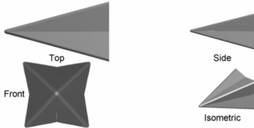
Figure 6.28: Vehicle D. Minimum maximum heat rate starbody waverider for M = 60 , Alt = 25 km. L/D = .122 , R = .199 m, \eta_V = 68.8\% , \dot{q}_{max} = 73.3 KW/cm 2 , \dot{q}_{net} = 221.7 KW, SM = -29.5\%
