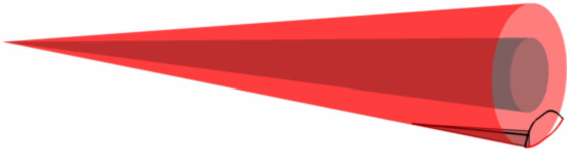
Figure 3.36: Trace of one streamline which will form the bottom waverider surface. Note that the waverider upper surface and shock have been translated and rotated so that the triangle formed in step 6 is entirely in the x-z plane.
